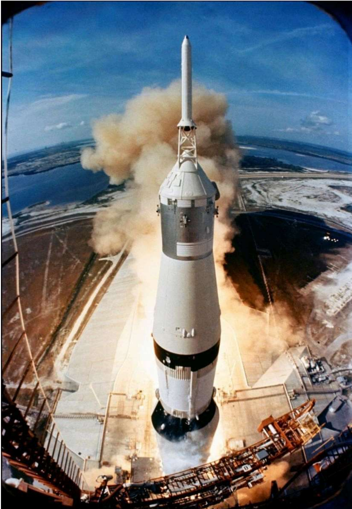
Apollo 11's Saturn V rocket liftoff. The Command Module, Service Module, and emergency escape tower are at the top. (The tower would carry the Command Module away during the launch and first few minutes of the flight, if the Saturn V exploded. The tower was jettisoned after only a few minutes into flight, if not used.) The Lunar Module is below the Service Module, protected by an outer, four-piece cover with conic, slanted sides. The LM sits on top of the third stage rocket of the
