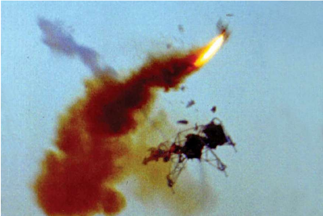
“Future moonwalker Neil Armstrong ejects [shown at top of image] from a Lunar Landing Research Vehicle (LLRV) after its control thrusters fail.” (Photo Credit: HistoryNet.com/NASA)
